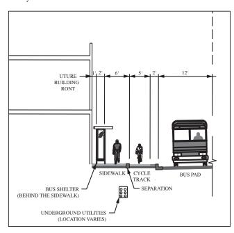
Potential sidewalk and cycle track configuration where bus pads may be provided.
